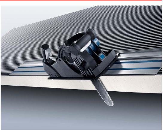
The new Panel Cutter TruTool 165 cuts polyurethane and polyisocyanurate Insulated Metal Panels regardless of whether the panel surface is flat, high rib or corrugated. The machine can handle diverse applications, ranging from crosscuts and right-angle cuts to interior cutouts and notches. Even cutouts on pre-mounted panels are easy work for the new panel cutter.
