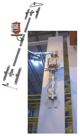
Using 4 x 440 lbs double suction pads, the lift capacity of the unit can be increased to 1760 lbs in defined configurations.
