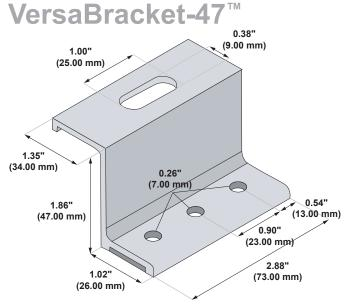
3 holes are provided for versatility. Some installations require only 2 fasteners. See the load table on the S-5! website and the installation instructions for more details.
